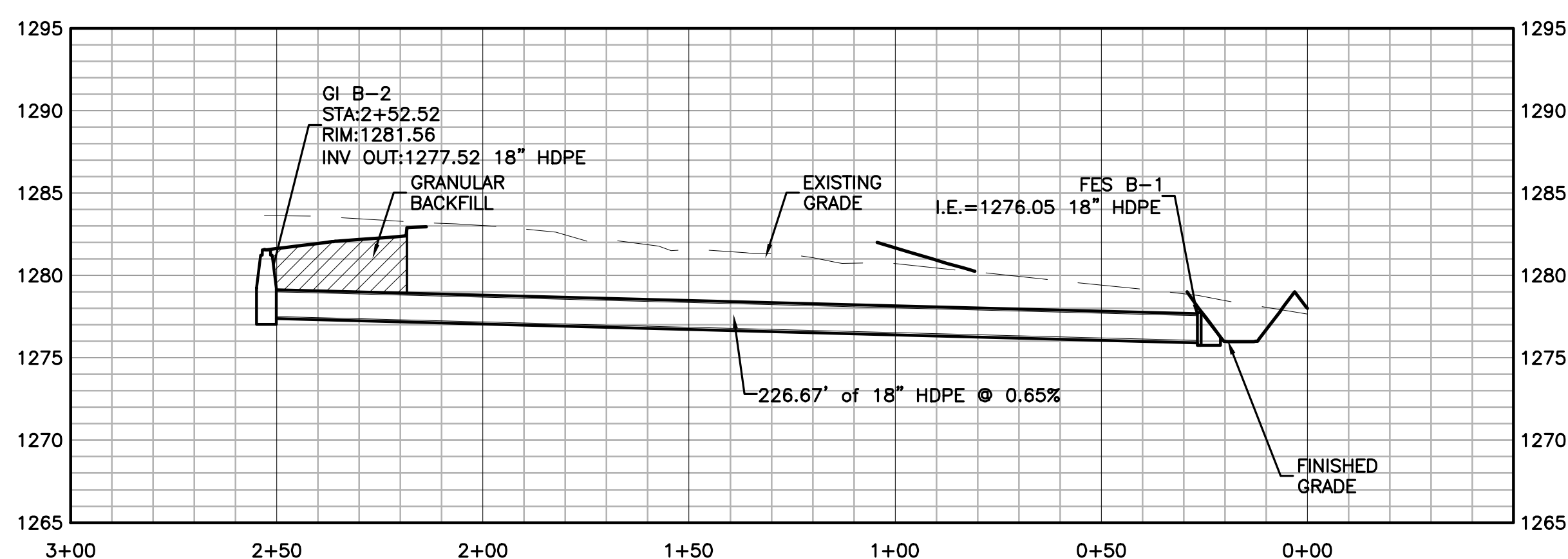
STORM SEWER LINE B HORIZONTAL SCALE: 1" = 30' VERTICAL SCALE: 1" = 5'
